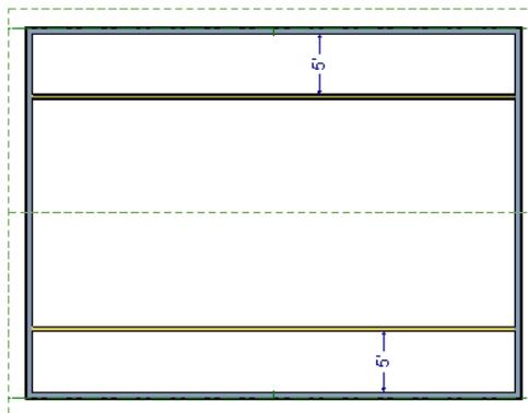
3. Select each of the interior walls one at a time and click the **Open Object**
