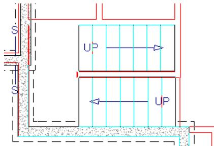
6. Select each stair section and adjust its width and position using its edit handles so that it fits within the walls forming the stairwell drawn on Floor 1.
