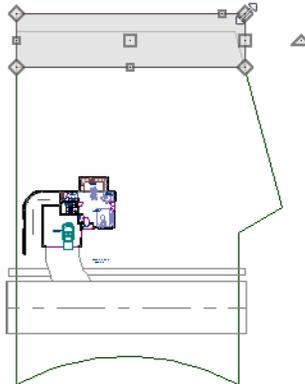
4. Select the Terrain Feature and click the **Open Object**
