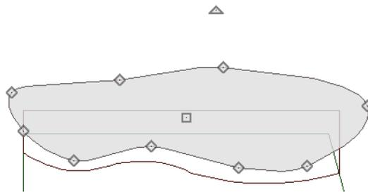
2. Select the pond and click the **Open Object**
