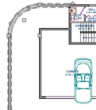
5. Draw two **Elevation Lines**
