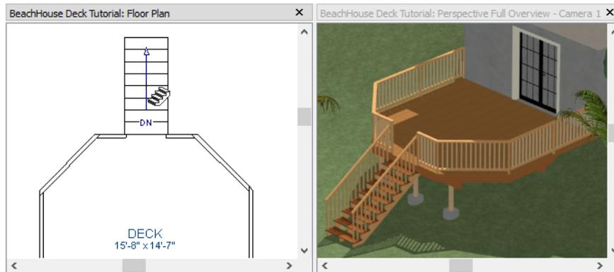
4. In most cases when using the **Click Stairs**
