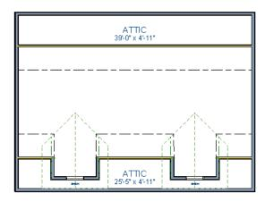
8. Select each of the knee walls and move them back so that they are in alignment with the ceiling plane. When **Object Snaps** are enabled, the walls will snap into position when they are close to the Ceiling Break Lines.
