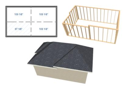
If you generate a roof and it seems to be more complicated and has more roof planes than it should, take a look at the ceiling heights of the rooms in the plan. Often, the correct way to create a lowered ceiling condition will be to set the ceiling at the default height create a lowered Ceiling Finish. See "Lowered Ceilings" on page 138 of the Reference Manual.
