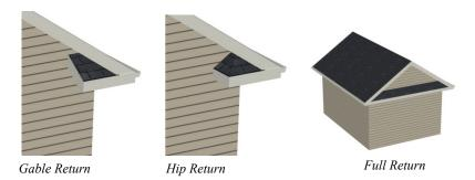
The first two are called **Gable** and **Hip** returns, since the returns themselves end in either a gable or a hip. The third is called a **Full** return because it extends under the entire gable, connecting both sides. Full roof returns are sometimes referred to as water tables.
