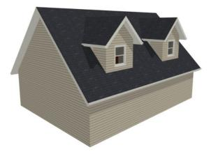
7. Notice that there are small gaps in the dormer side walls. This gap is caused by the difference between the position of the knee walls and the point at which the ceiling intersects the roof plane. This location is marked by the black dotted Ceiling Break Line in plan view.
