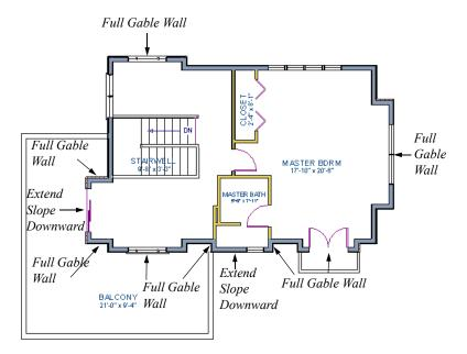
7. Once these roof directives have been assigned, the roof can be generated.
