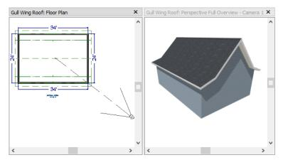
Experiment with the height at which the second pitch begins so that you can see the effect it has on the gull wing roof design.
