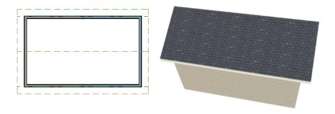
If a wall that is perpendicular to these walls is also specified as a Full Gable Wall, the roof becomes more complex with an additional ridge, two valleys, and two hips.
