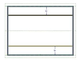
3. Select each of the interior walls one at a time and click the **Open Object** ledit button. Check the box beside **Knee Wall** on the ROOF panel of the **Wall Specification** dialog and click **OK**.
