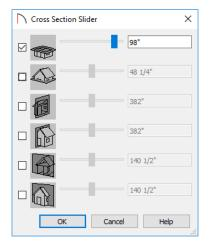
5. Select the horizontal cut line and use the **Position** slider to specify the location of the cutting plane. See "Cross Section Slider" on page 419 of the Reference Manual.
