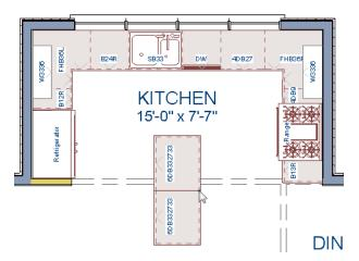
In the next portion of this tutorial, the display of cabinet labels is turned off. To do this, select **Tools> Display Options** . In the **Display Options** dialog, locate the "Cabinets, Labels" layer, remove the check mark in the **Disp** column, and click **OK**.
