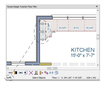
When objects are very close to one another in floor plan view, it may be difficult to select the intended object. When an object is selected, click the Select Next Object edit button or press the Tab key to select a nearby object. See "Select Next Object" on page 87 of the Reference Manual.
