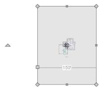
In addition to adjusting the size of your rectangular Terrain Perimeter, you can also use the **Change Line/Arc**  $\ \ \ \ \ \$  and **Break Line**  $\ \ \ \ \$  edit tools to modify its shape.
