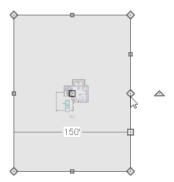
2. You can then use the new edit handles to adjust the size and shape of the Terrain Perimeter. For more information, see "Editing Closed-Polyline Based Objects" on page 92 of the Reference Manual.
