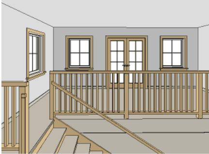
To produce a break in a railing for a stairway or other access, use a **Doorway**
