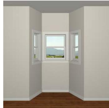
Both the top and bottom heights of these window units can be adjusted in a 3D view using the window's edit handles to create a lowered ceiling and/or a bench seat or garden window.
