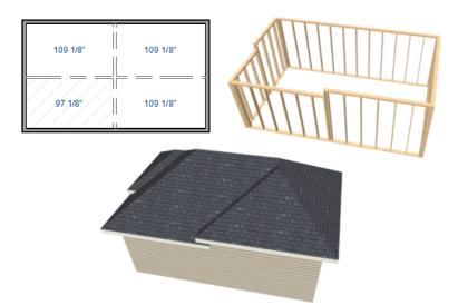
If you generate a roof and it seems to be more complicated and has more roof planes than it should, take a look at the ceiling heights of the rooms in the plan. Often, the correct way to create a lowered ceiling condition will be to set the ceiling at the default height create a lowered Ceiling Finish. See "Lowered Ceilings" on page 240 of the Reference Manual.
