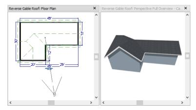
The gable wall on the left produces roof planes that extend too high and interfere with the roof over the front extension of the house. To avoid this, use the Break edit tool to divide the left wall into two different sections. The upper section can then be specified as a Full Gable without affecting the lower section.
