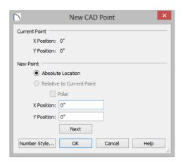
2. Select **Absolute Location** and define the point's position at (0,0) and click **OK**. This is the current point that serves as the Start Point for the first line of the plot plan. See "Point Tools" on page 165 of the Reference Manual.
