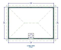
• Midpoint Object Snaps or the Center Objects edit tool can be used to center the fireplace along the wall, if desired. See "Using Center Object" on page 193 of the Reference Manual.
