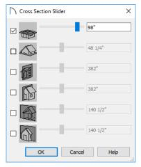
5. Select the horizontal cut line and use the **Position** slider to specify the location of the cutting plane. See "Cross Section Slider" on page 784 of the Reference Manual.
