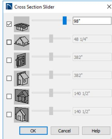
5. Select the horizontal cut line and use the **Position** slider to specify the location of the cutting plane. See “Cross Section Slider” on page 784 of the Reference Manual.
