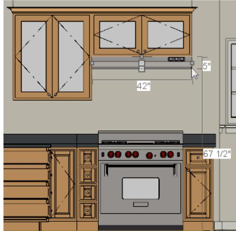
Dimensions can be added to objects displayed in Cross Section/Elevation views, including cabinetry. To begin, return to your Floor Plan view, if you haven't already.
