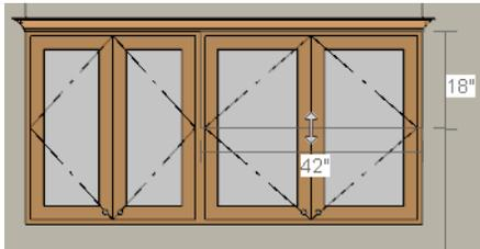
3. When the temporary dimension indicates that the cabinet height is 18 inches, release the mouse button.
