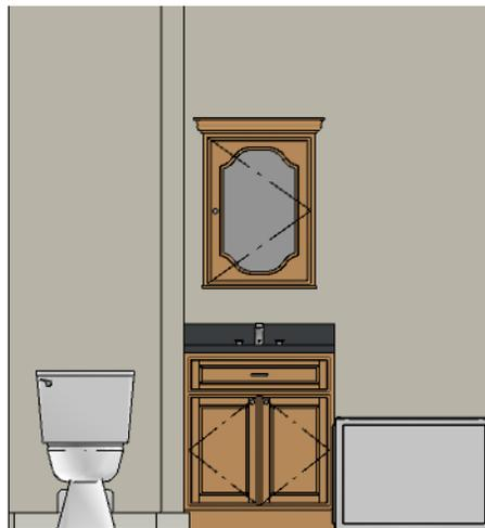
1. On Floor 2, select **3D> Create Orthographic View> Wall Elevation**
