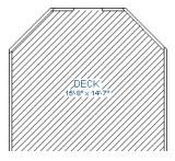
5. When deck planking is displayed in floor plan view and you wish to select the Deck room, you will most likely select a plank instead. When this happens, click the Select Next Object edit button or press the Tab key until the room is selected.
