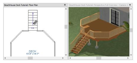
4. In most cases when using the **Click Stairs** tool, an opening will be added automatically to the deck railing at the top of a staircase.
