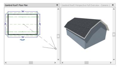
Experiment with alternate pitches and overhangs. Also, try varying the height at which the second pitch begins so that you can see the effect it has on the gambrel roof design.
