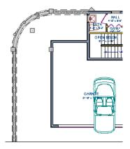
5. Draw two **Elevation Lines** just inside the retaining wall to define the height of this area when terrain is generated. These Elevation Lines can stay at their default height of 0".
