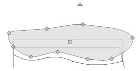
2. Select the pond and click the **Open Object** dedit button. On the GENERAL panel of the **Terrain Feature Specification** dialog, raise the **Height** to 1 inch. This will position the water material above the beach.
