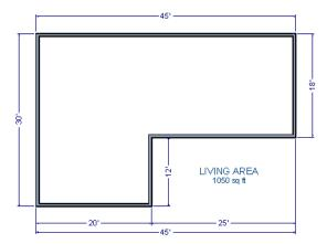
To create a reverse gable in this plan, three gable walls are required: two running vertically and one horizontally.
