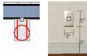
Wall-mounted outlet in 2D and 3D views
