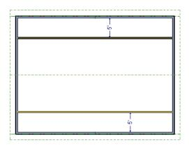
3. Select each of the interior walls one at a time and click the **Open Object** edit button. Check **Knee Wall** on the Roof tab of the **Wall Specification** dialog and click OK.
