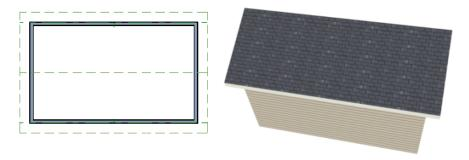
If a bumpout is added that affects the length of either Full Gable Wall, or if an alcove is added anywhere along the length of the structure, the ridge will no longer follow a straight line.
