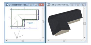
Built this way, the gable wall on the left produces roof planes that extend too high and will interfere with the roof over the lower part of the house. To correct this, use the **Break Wall**
