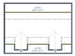
8. Select each of the knee walls and move them back so that they are in alignment with the ceiling plane. The walls will snap into position when they are close to the ceiling lines.
