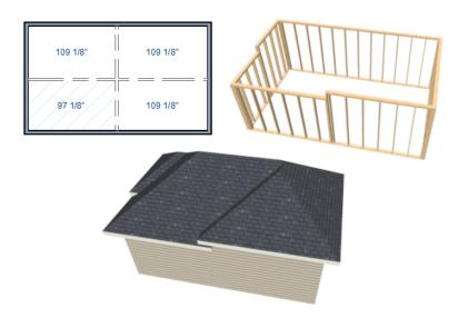
If you generate a roof and it seems to be more complicated and has more roof planes than it should, take a look at the ceiling heights of the rooms in the plan. Often, the correct way to create a lowered ceiling condition will be to set the ceiling at the default height create a lowered Ceiling Finish. See "Lowered Ceilings" on page 125 of the Reference Manual.
