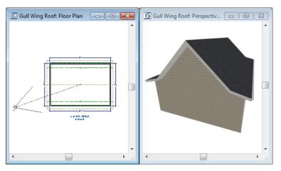
Experiment with the height at which the second pitch begins so that you can see the effect it has on your gull wing roof design.
