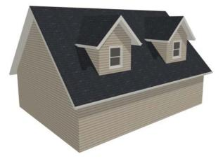
You can move the interior walls closer to or further from the outside walls to change the dormers' elevation, or change the pitch for the roof to make the dormers longer. You can create dormers in more complex plans the same way, but you may want to experiment with wall placement and pitch to achieve the desired effect.
