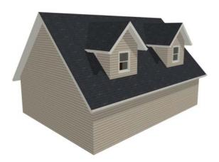
7. Notice there are small gaps in the dormer side walls. This gap is caused by the difference between the position of the knee walls and the point at which the ceiling intersects the roof plane. This location is marked by the black dotted line in floor plan view.
