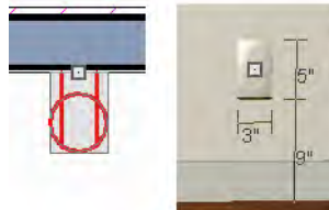
Wall-mounted outlet in 2D and 3D views
