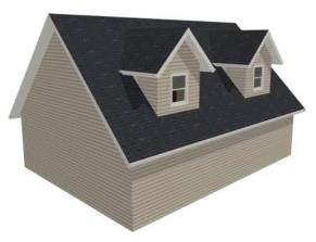
7. Notice that there are small gaps in the dormer side walls. This gap is caused by the difference between the position of the knee walls and the point at which the ceiling intersects the roof plane. This location is marked by the black dotted Ceiling Break Line in floor plan view.
