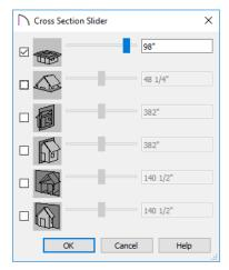
5. Select the horizontal cut line and use the **Position** slider to specify the location of the cutting plane. See "Cross Section Slider" on page 395 of the Reference Manual.
