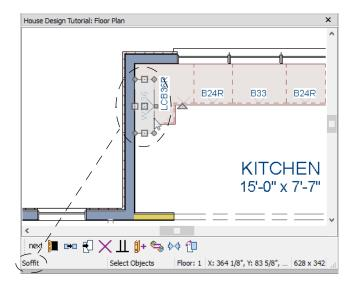
When objects are very close to one another in floor plan view, it may be difficult to select the intended object. When an object is selected, click the Select Next Object edit button or press the Tab key to select a nearby object. See "Select Next Object" on page 95 of the Reference Manual.
