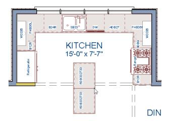
In the next portion of this tutorial, the display of cabinet labels is turned off. To do this, select **Tools> Display Options** . In the **Display Options** dialog, locate the "Cabinets, Labels" layer, remove the check mark in the **Disp** column, and click **OK**.
