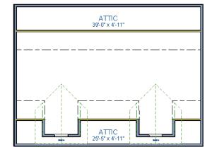
8. Select each of the knee walls and move them back so that they are in alignment with the ceiling plane. When **Object Snaps** are enabled, the walls will snap into position when they are close to the Ceiling Break Lines.
