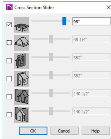
5. Select the horizontal cut line and use the **Position** slider to specify the location of the cutting plane. See “Cross Section Slider” on page 387 of the Reference Manual.
