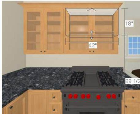
3. When the temporary dimension indicates that the cabinet height is 18 inches, release the mouse button.
