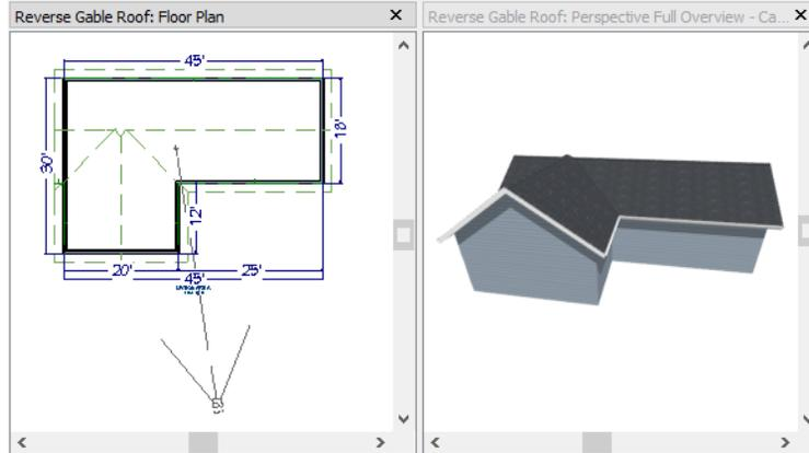
Notice the step in the ridge line. This can be corrected by resizing the lower gable wall. Select the vertical wall to the right of the bottom gable wall and move it to the left 2 feet, reducing the length of the gable wall from 20 to 18 feet. When you are finished, rebuild the roof.
