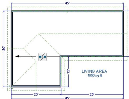
2. Open the lower portion of the wall for specification and on the **ROOF** panel of the **Wall Specification** dialog, clear the **Full Gable Wall** checkbox and click **OK**.
