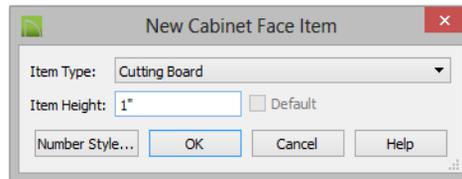
5. Select "Cutting Board" from the **Item Type** drop-down list, assign an **Item Height** of 1 inch and click **OK** to return to the **Cabinet Specification** dialog.
