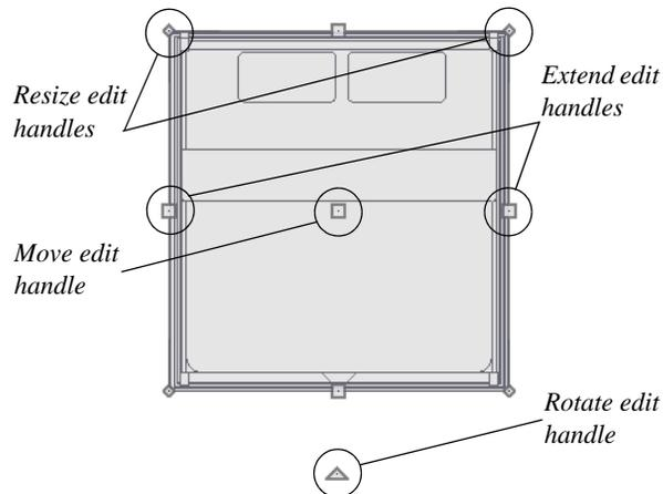
2. Use the Rotate edit handle to rotate the bed.
