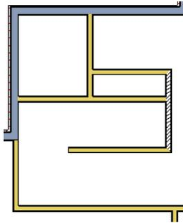
4. Draw a horizontal **Interior Dimension**
