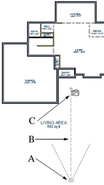
4. Release the mouse button to create the 3D camera view. Where the mouse is released (C) is the camera's focal point.
