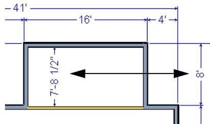
Note: Interior Dimensions locate the framing layer of walls by default rather than wall surfaces.
