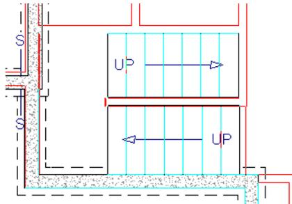
6. Select each stair section and adjust its width and position using its edit handles so that it fits within the walls forming the stairwell drawn on Floor 1.
