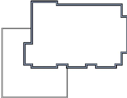
5. If **Object Snaps**
