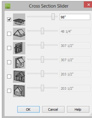
5. Select the horizontal cut line and use the **Position** slider to specify the location of the cutting plane. See “Cross Section Slider” on page 339 of the Reference Manual.
