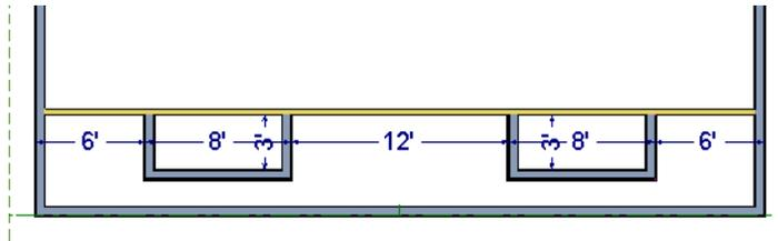
2. Position the front walls of each dormer box 2 feet from the bottom exterior wall. The front dormer walls are those parallel to the bottom wall.
