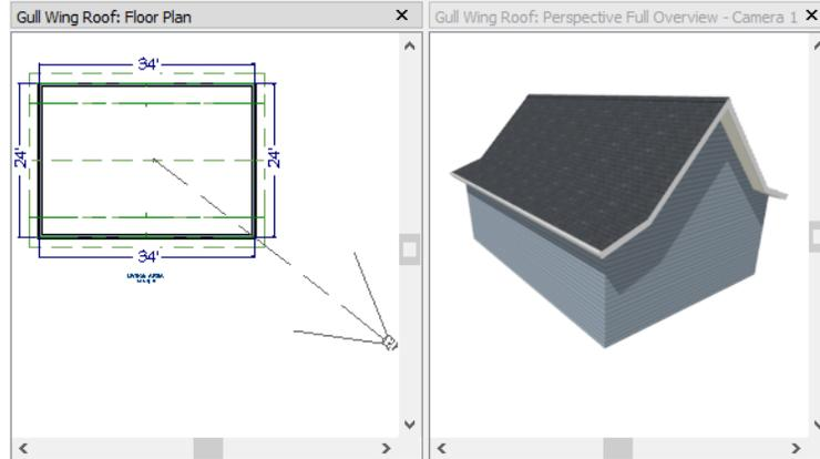
Experiment with the height at which the second pitch begins so that you can see the effect it has on the gull wing roof design.
