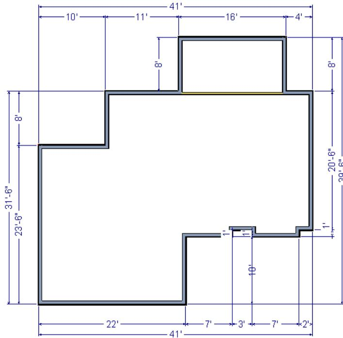
Dimensions can also be used to change the length of a selected wall. Bear in mind, though, that the when a wall is resized in this manner its Start point will always be locked and its End point will always be moved. Because of this, it is often easier to move walls than to resize them. See “Editing Walls” on page 122 of the Reference Manual.
