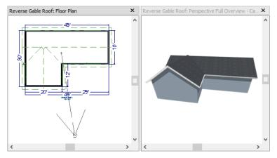
Notice the step in the ridge line. This can be corrected by resizing the lower gable wall. Select the vertical wall to the right of the bottom gable wall and move it to the left 2 feet, reducing the length of the gable wall from 20 to 18 feet. When you are finished, rebuild the roof.
