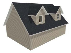
7. Notice that there are small gaps in the dormer side walls. This gap is caused by the difference between the position of the knee walls and the point at which the ceiling intersects the roof plane. This location is marked by the black dotted Ceiling Break Line in floor plan view.
