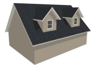
You can move the interior walls closer to or further from the outside walls to change the dormers' elevation, or change the pitch for the roof to make the dormers longer. You can create dormers in more complex plans the same way, but you may want to experiment with wall placement and pitch to achieve the desired effect.
