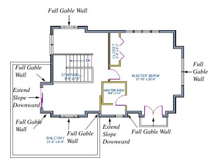
7. Once these roof directives have been assigned, the roof can be generated.
