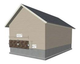
Soffits automatically stop at the floor platform when moved downward or at the ceiling platform when moved upward - even when the soffit is not located in a room. To more or resize a soffit through a floor or ceiling platform, select it and hold the Ctrl key down while dragging its edit handles. See "Unrestricted Movement" on page 99.
