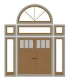
Notice how the windows and door in this example are separate, with spaces between them. Doors and/or windows can also be organized into a unit in which there are no spaces between the windows and door units, and the casing between them is shared.
