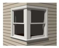
To create a corner window, first create the desired window on each side of the corner. The header height and the sill height of both windows must be the same.
