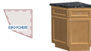
Left End Cabinet
