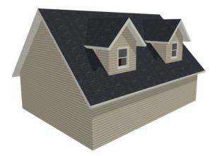
7. Notice that there are small gaps in the dormer side walls. This gap is caused by the difference between the position of the knee walls and the point at which the ceiling intersects the roof plane. This location is marked by the black dotted Ceiling Break Line in plan view.
