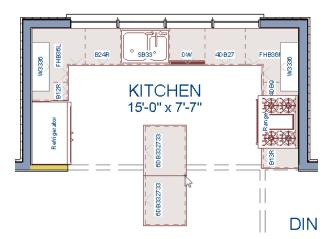
In the next portion of this tutorial, the display of cabinet labels is turned off. To do this, select **Tools> Display Options** . In the **Layer Display Options** dialog, locate the "Cabinets, Labels" layer, remove the check mark in the **Disp** column, and click **OK**.
