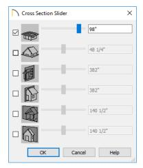
5. Select the horizontal cut line and use the **Position** slider to specify the location of the cutting plane. See "Cross Section Slider" on page 475 of the Reference Manual.
