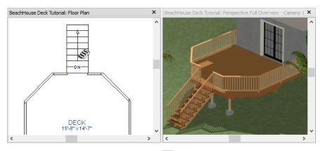
4. In most cases when using the **Click Stairs** tool, an opening will be added automatically to the deck railing at the top of a staircase.
