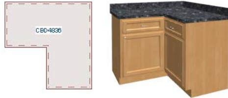
Corner cabinet with sides of equal width
