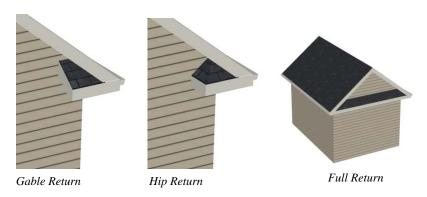
The first two are called **Gable** and **Hip** returns, since the returns themselves end in either a gable or a hip. The third is called a **Full** return because it extends under the entire gable, connecting both sides. Full roof returns are sometimes referred to as water tables.
