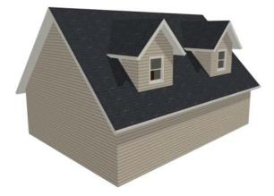
7. Notice that there are small gaps in the dormer side walls. This gap is caused by the difference between the position of the knee walls and the point at which the ceiling intersects the roof plane. This location is marked by the black dotted Ceiling Break Line in floor plan view.
