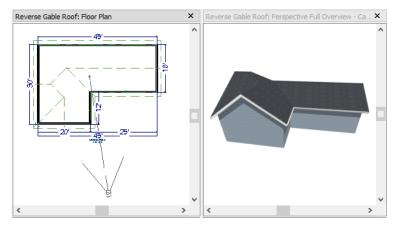
The gable wall on the left produces roof planes that extend too high and interfere with the roof over the front extension of the house. To avoid this, use the Break Wall tool to divide the left wall into two different sections. The upper section can then be specified as a Full Gable without affecting the lower section.
