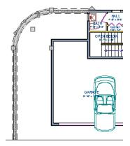
5. Draw two **Elevation Lines** just inside the retaining wall to define the height of this area when terrain is generated. These Elevation Lines can stay at their default height of 0".
