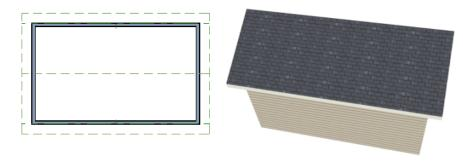
If a bump out is added that affects the length of either Full Gable Wall, or if an alcove is added anywhere along the length of the structure, the ridge will no longer follow a straight line.
