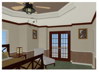
3. Click once on the crown molding to load the wood material. Notice that the mouse pointer changes to a spray can <sup>+</sup>, indicating that the loaded material is ready to apply to another object.
