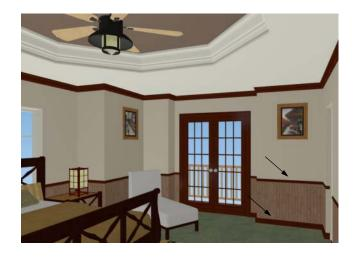
4. Click on the chair rail and base moldings to apply the loaded material.
