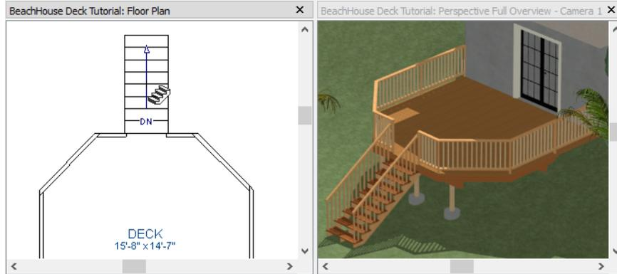
4. In most cases when using the **Click Stairs**
