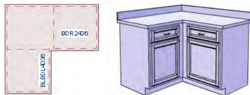
Two base cabinets and the filler between them
